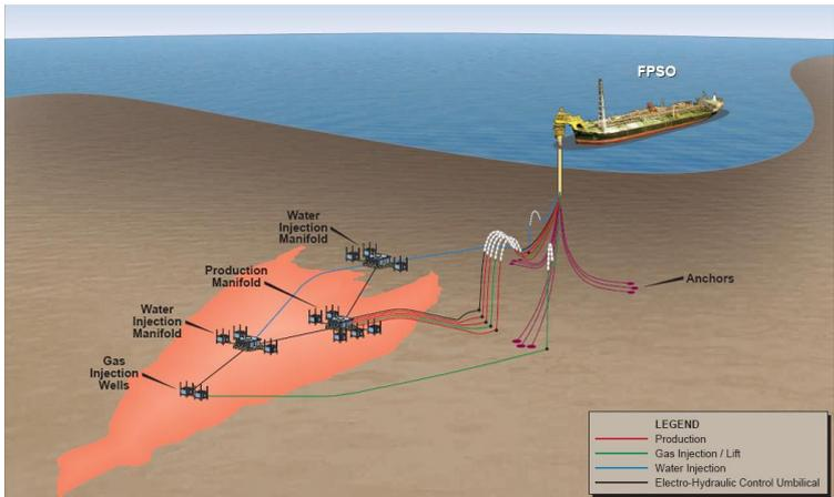
In Western Australia and the Northern Territory, oil installations frequently feature subsea wells with control and isolation equipment located on the seabed. Generally, oil is stored in oil tankers converted to production facilities called an “FPSO” or floating production, storage and offtake vessels. Gas is generally piped to shore from these facilities depending on the quantities involved.
